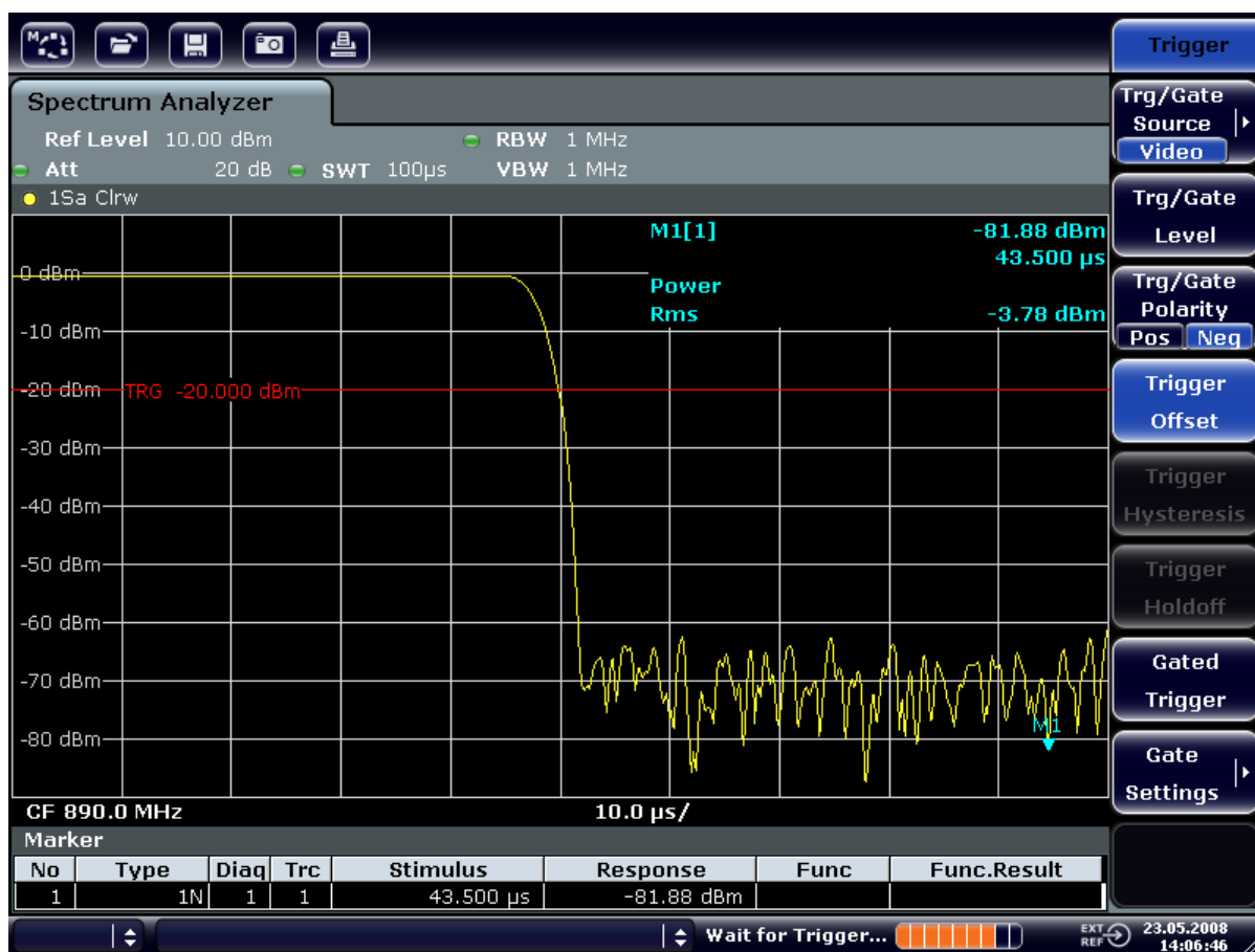
Figure 3-17: Falling edge of the GSM burst displayed with high time resolution
