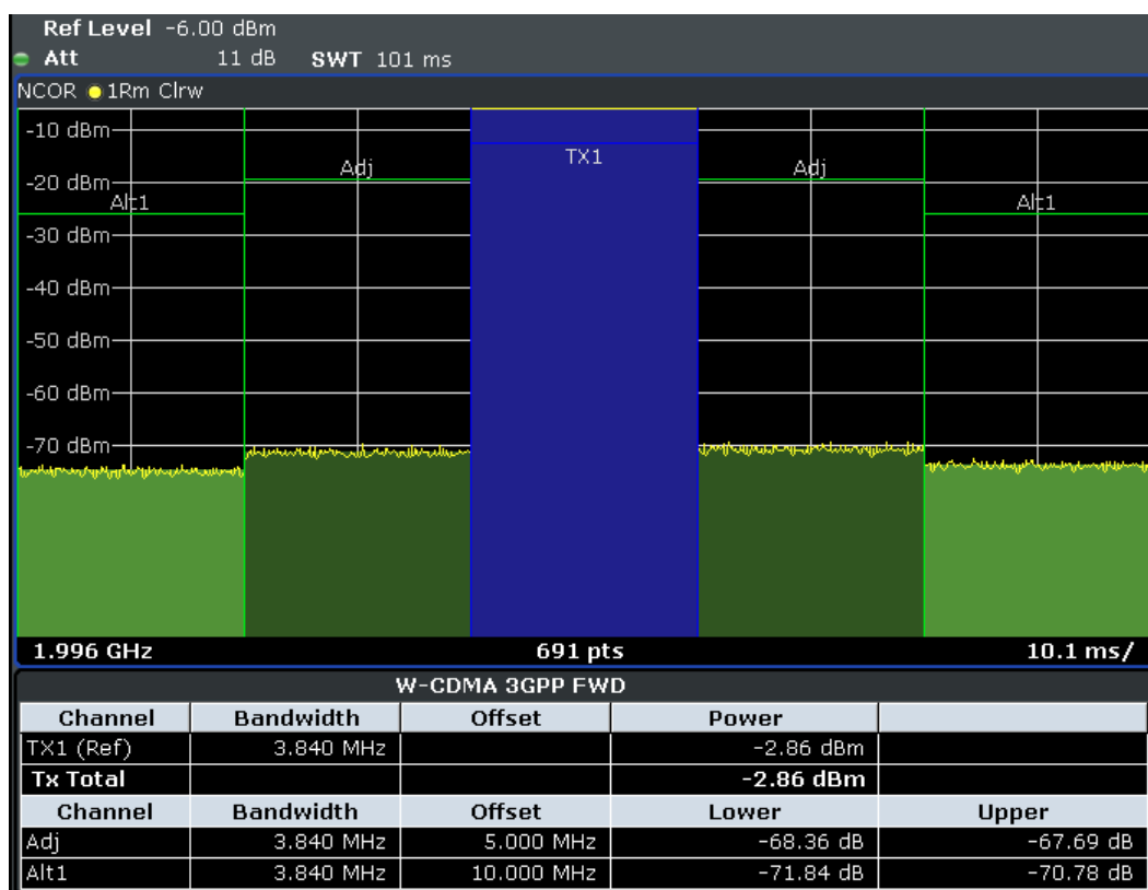
Figure 6-34: Measuring the adjacent channel power of a W-CDMA signal with the fast ACLR mode
