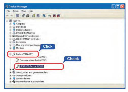
Check the COM number to the right of "HIOKI USB Device" in the [Ports (COM & LPT)] list.
