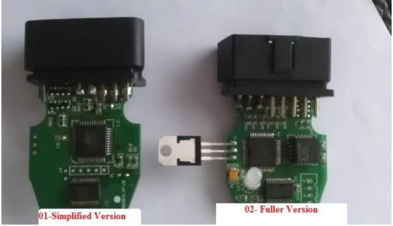
Pictures above are Vag 12.10's Circuit Boards, Picture No.1 is Hardware Circuit in Simplified Version, while Picture No.2 is in Fuller Version. Fuller Version contains 2 more ICs and Peripheral electronic components, works much more stable than Simplified Version.
