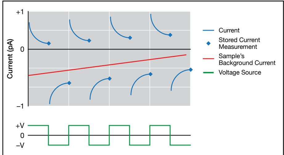
The alternating voltage source polarity method eliminates the effects of background currents in materials for making repeatable, accurate high resistance and resistivity measurements.
