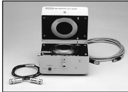
**8009 Resistivity Chamber is compliant with American Society for Testing and Materials (ASTM) Standard D 257 Standard Test Methods for DC Resistance or Conductance of Insulating Materials. The 8009 combined with the 6517B provides a complete system for making high quality, safe resistivity measurements.**
