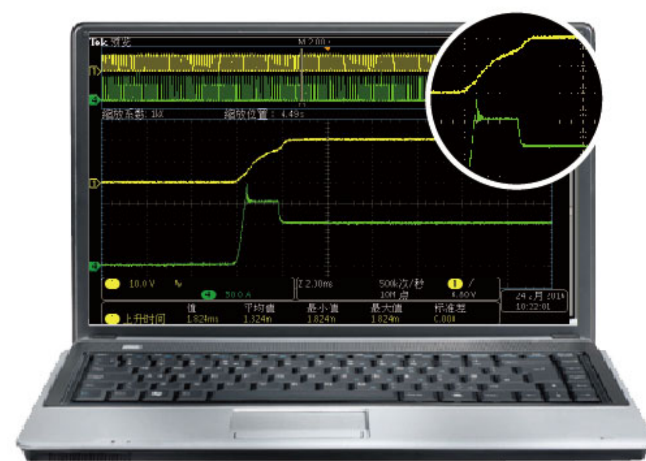
启动浪涌电流超电流量程，高速建立电压 (CV-High, CC-Low, CV优先)
