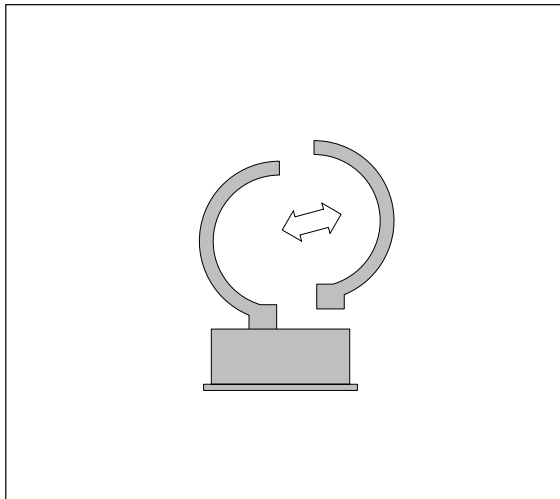
3. Remove one antenna segment
