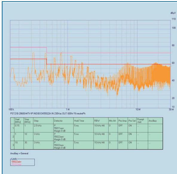
According to EN55022A IN 230Vac OUT 600V Phase for PST21B-28600-MTV-IP
