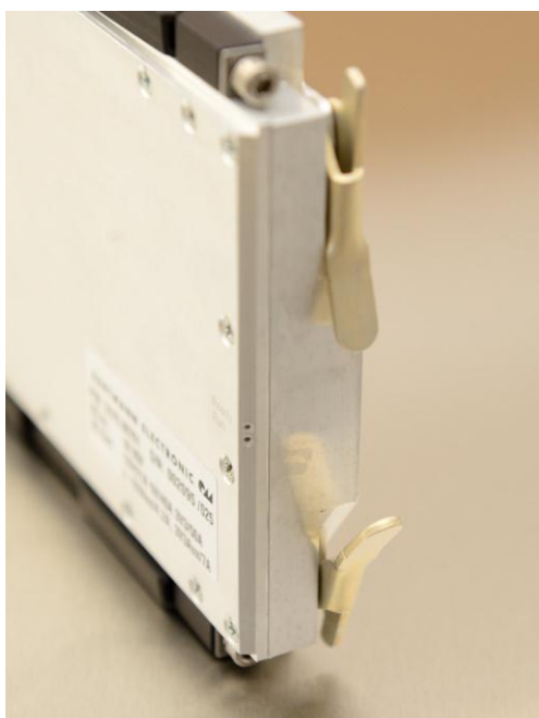
Figure 2 Front panel functional elements of the VPX3C Power Supply
