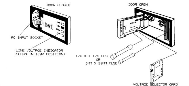
Figure 2-3. Line Module Detail
