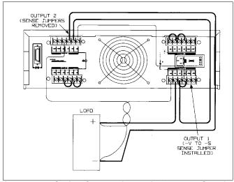
Figure 4-14. Series Connections with Remote Sensing
