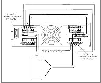
Figure 4-11. Parallel Connections with Local Sensing
