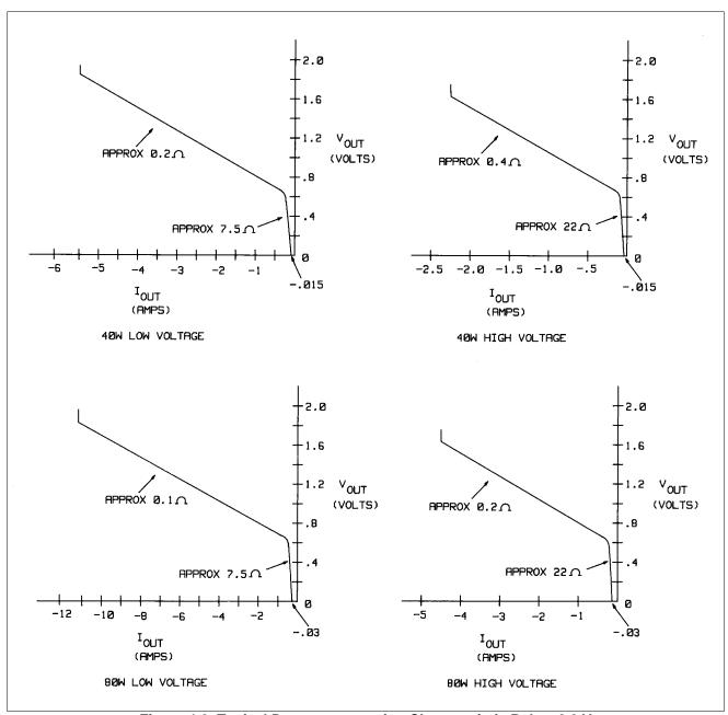
Figure 4-3 Typical Downprogramming Characteristic Below 2.0 V
