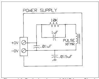
Figure 4-9. Equivalent Internal OV Trigger Circuit
