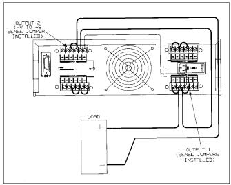
Figure 4-13. Series Connections with Local Sensing
