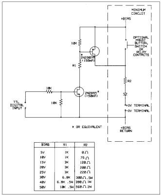
Figure 4-8. External Trigger Circuit
