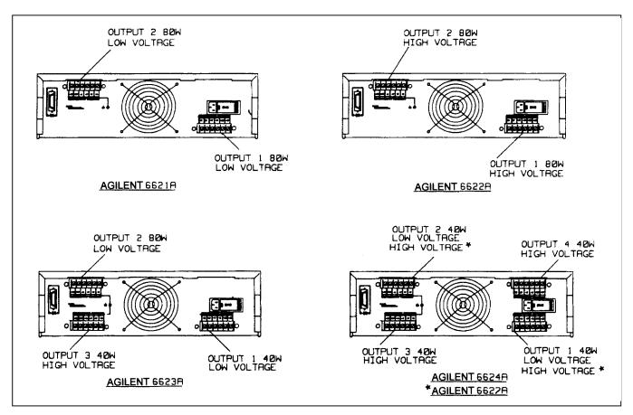
Figure 4-1. Output Connections
