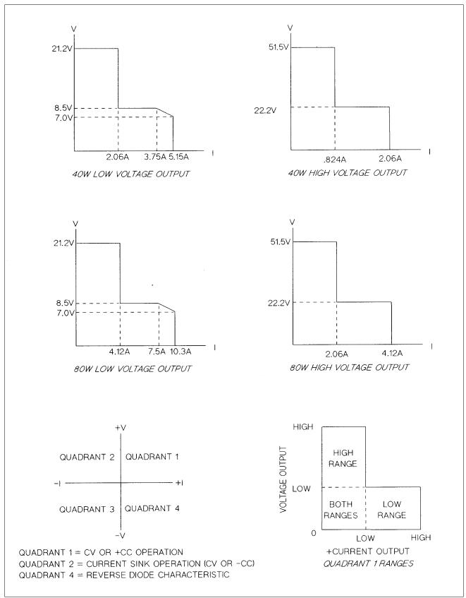
Figure 4-2. Typical Output Range Characteristics
