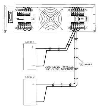
Figure 4-4. Optimum Hookup for Multiple Loads, Local Sensing
