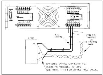
Figure 4-5. Remote Voltage Sensing
