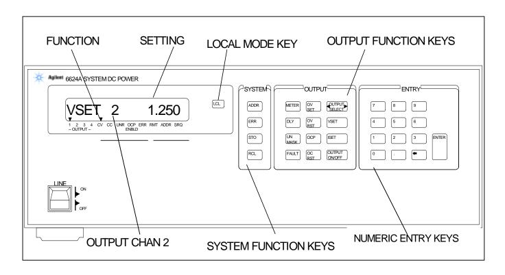
Figure 6-1. Front Panel (Model 6624A shown)
