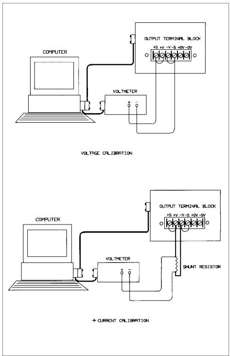
Figure A-1. Calibration Setup
