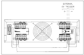
Figure 4-7. Overvoltage Connections
