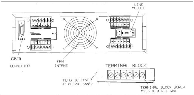
Figure 2-2. Rear Panel Detail (6624A Shown)
