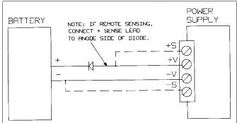
Figure 4-10. Recommended Protection Circuit for Battery Charging
