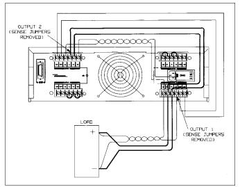
Figure 4-12. Parallel Connections with Remote Sensing
