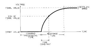
Figure 1-3. Output Response Characteristics
