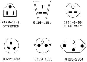
Figure 2-4. Power Cord Plug Configurations
