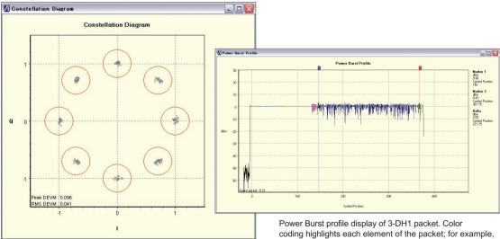
BlueSuite Pro3 displays the IQ constellation pattern for all payload symbols, or any user defined 50 µs block. Limit circles are preset to the core specification requirement for  $\pi/4DQPSK$  or 8DPSK modulation standards
