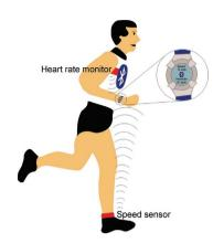
*Bluetooth* low energy wireless technology is the latest addition to the *Bluetooth* specification. It is designed specifically for small, button-cell battery powered devices for which low power-consumption and low cost are the primary concerns. *Bluetooth* low energy is designed to work side by side with existing *Bluetooth* devices. It operates in the 2.4 GHz ISM band and offers data rates of 1 Mbit/sec over a range of over 10 meters.
