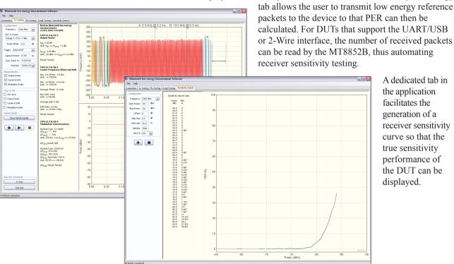
A dedicated tab in the application facilitates the generation of a receiver sensitivity curve so that the true sensitivity performance of the DUT can be displayed.
