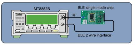
For DUT transmitter tests, test controls sent from the MT8852B configure the low energy device to transmit test reference packets that are captured and analyzed by the MT8852B receiver.
