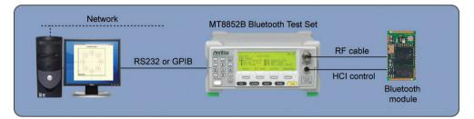
For fault finding and analysis, BlueSuite Pro3 software is a PC based tool kit that tests EUTs systematically on all channels. BlueSuite Pro3 also graphically displays the essential waveforms of power burst profile, modulation deviation and IQ diagrams.
