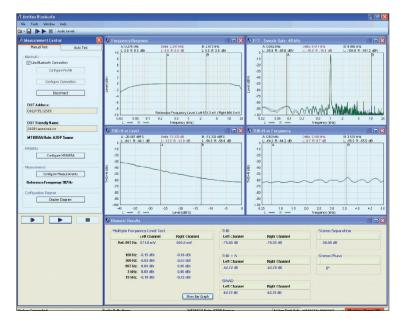
The BlueAudio software, supplied with each MT8855A, is installed on a PC that connects to the MT8855A using a standard USB cable. BlueAudio serves as the MT8855A's front panel and is used to configure the instrument and display graphical and numeric measurement results. It communicates with the MT8855A by means of the class library dll file.
