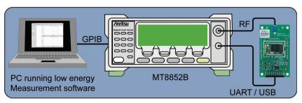
The MT8852B low energy PC application displays the power burst profile and modulation against symbol of low energy test reference packets. This is an invaluable tool during the design verification process for viewing and fully characterising the performance of a BLE radio.
