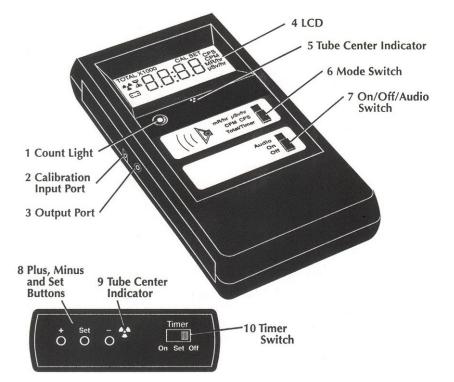
The palmRAD 907 counts ionizing events and displays the results on the liquid crystal display (LCD) (4). You control which unit of measurement is shown by using the mode switch.
