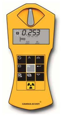
GAMMA-SCOUT® has an integrated quartz clock whose display can be activated by a pushbutton. Time and date are used to register the measured radiation. With a function in the data reading program of the TOOLBOX software, the GAMMA-SCOUT® date and time can be synchronized to the PC. Choose the menu "Set any time" to set your choice of date and time (i.e. different time zones) on the GAMMA-SCOUT®
