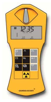
GAMMA-SCOUT® is powered by a Lithium Thionyl Chloride cell of 2.7 - 3.7 voltage. The device will continue functioning until the cell voltage is down to 2.8. When the voltage drops below this value, the battery symbol will appear in the display. The data will be retained, even at total breakdown of voltage. The model RECHARGEABLE has a rechargeable power supply (via USB or power supply unit that is included in delivery)
