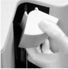
**Fig. 12. Remove light housing.**
