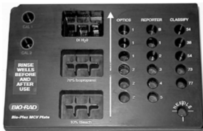
Fig. 6. Maintenance, calibration and validation (MCV) plate.
