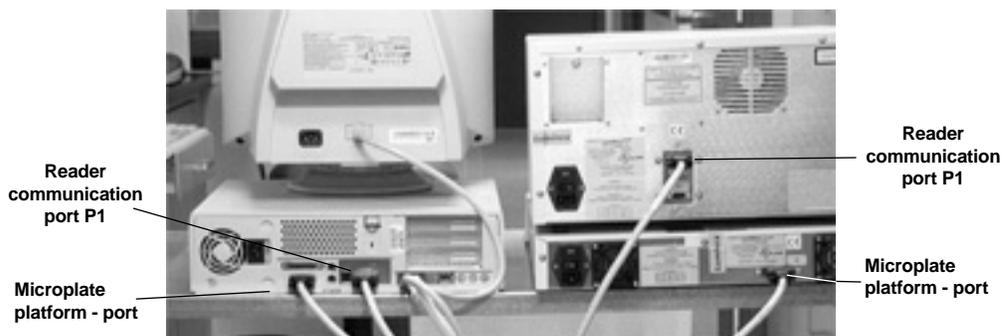
Fig. 11. Completed connections of computer and monitor to the Bio-Plex protein array system.
