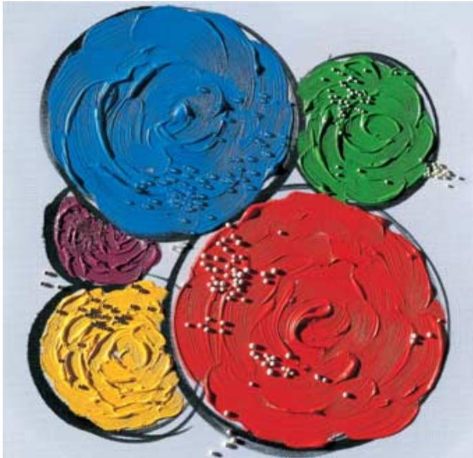
In many technical processes it is necessary to divide solid material into fine particles and distribute them evenly within a liquid carrier. This process is generally known as "dispersion".
