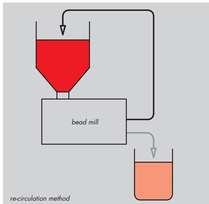
schematic view of pass and re-circulation method
