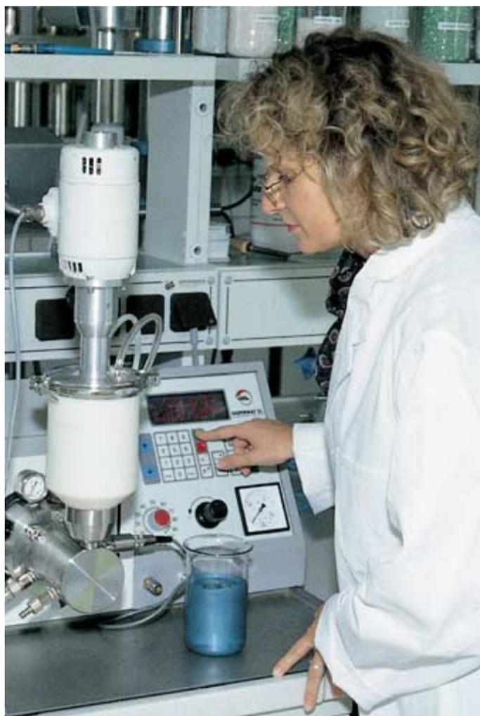
It does not matter whether the power input which leads to the existing energy density, is applied with a high speed and low torque or vice versa. With a given bead charge and dispersion time, the dispersion result depends only on the amount of the mechanical power.
