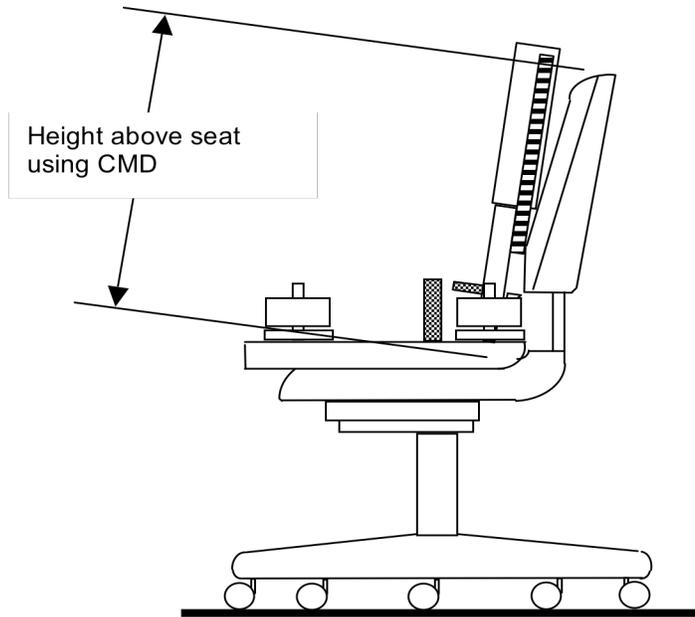
**Figure 15a - Test Height Determination
