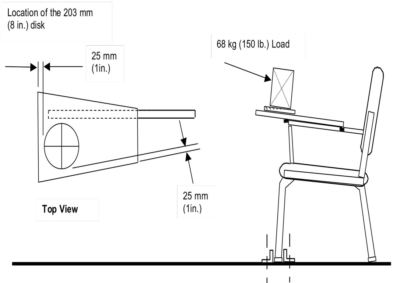
Figure 23 - Tablet Arm Chair Static Load Test
