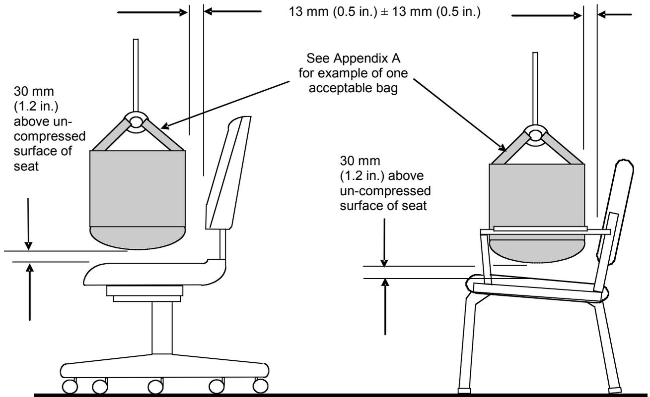
Figure 11a - Seating Durability Test - Cyclic
