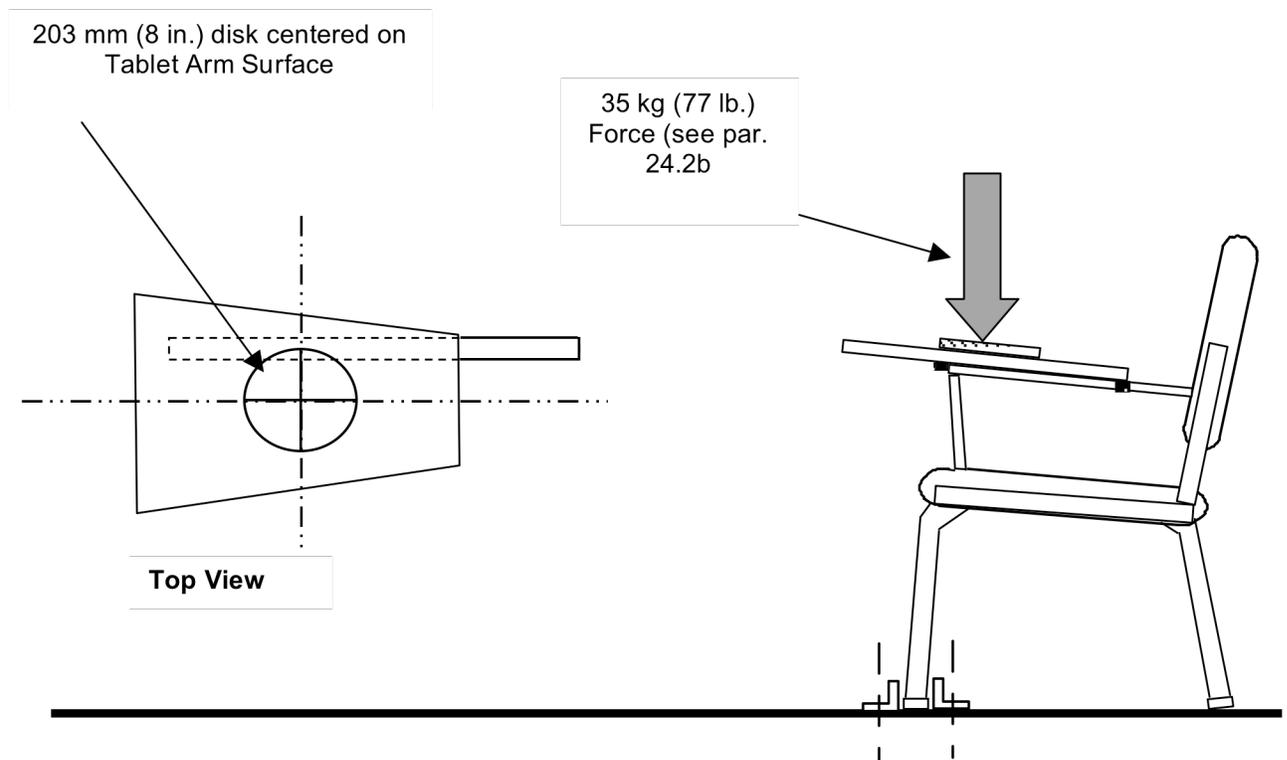
Figure 24 - Tablet Arm Chair Load Ease Test - Cyclic
