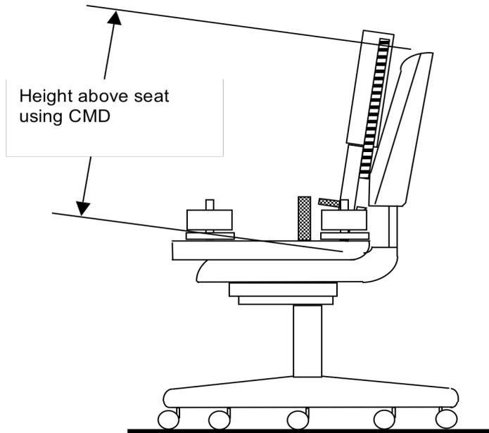
**Figure 16a - Test Height Determination
