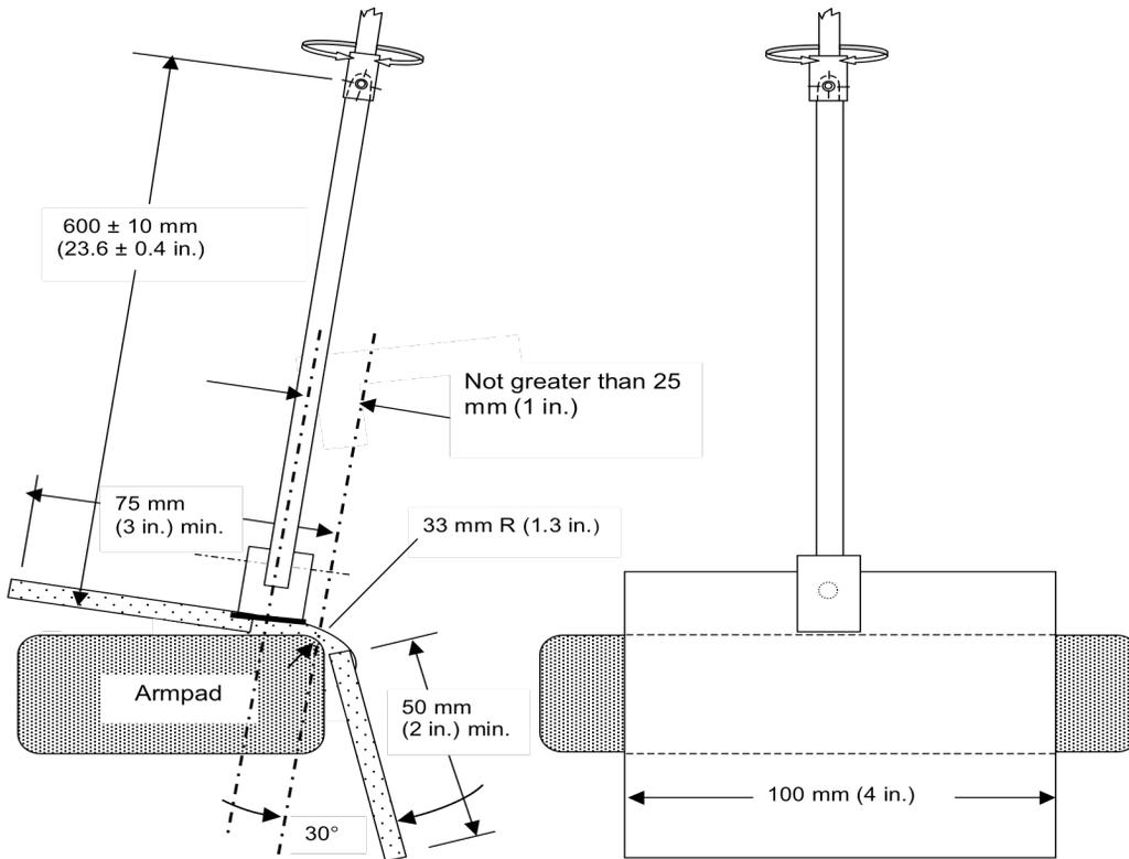
Figure 21a - Arm Loading Device
