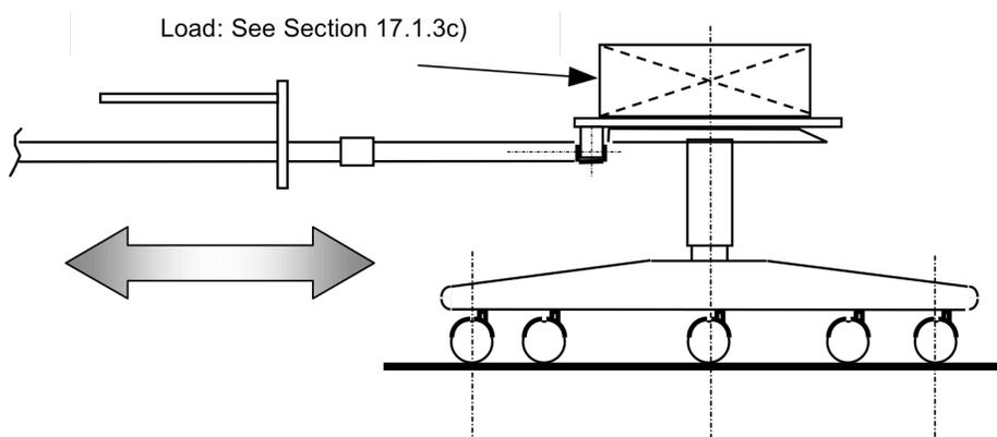
Figure 17c - Machine Schematic for Pedestal Base Chairs
