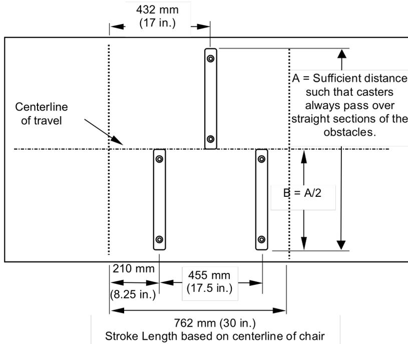
Figure 17b - Obstacle Layout for Pedestal Base Chairs
