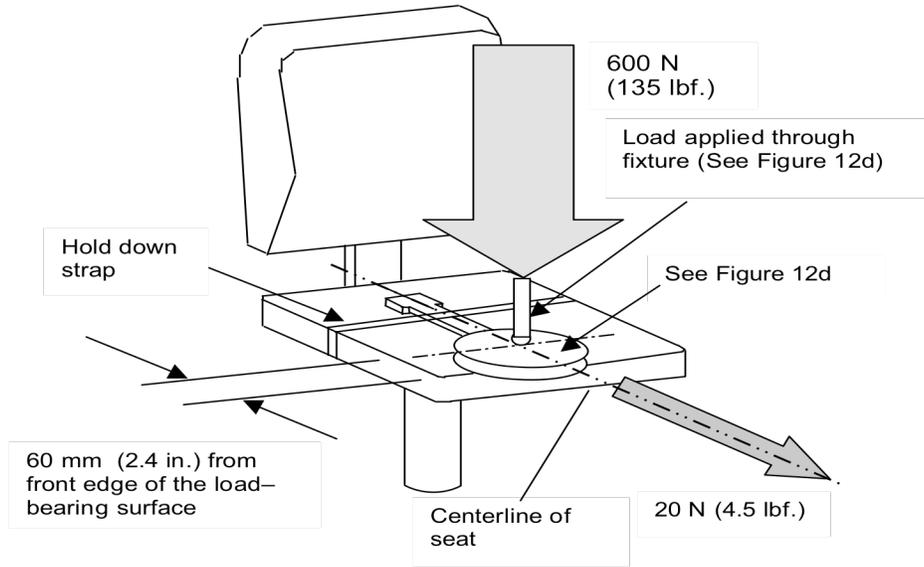
Figure 12c - Front Stability Test
