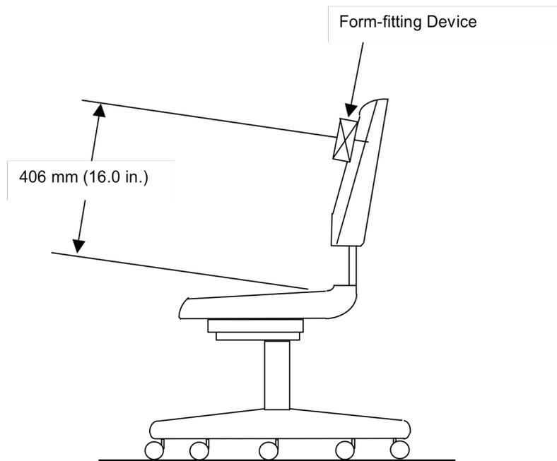
**Figure 16b - Positioning of Form-Fitting Device for Backrests Higher than 452 mm (17.8 in.)
