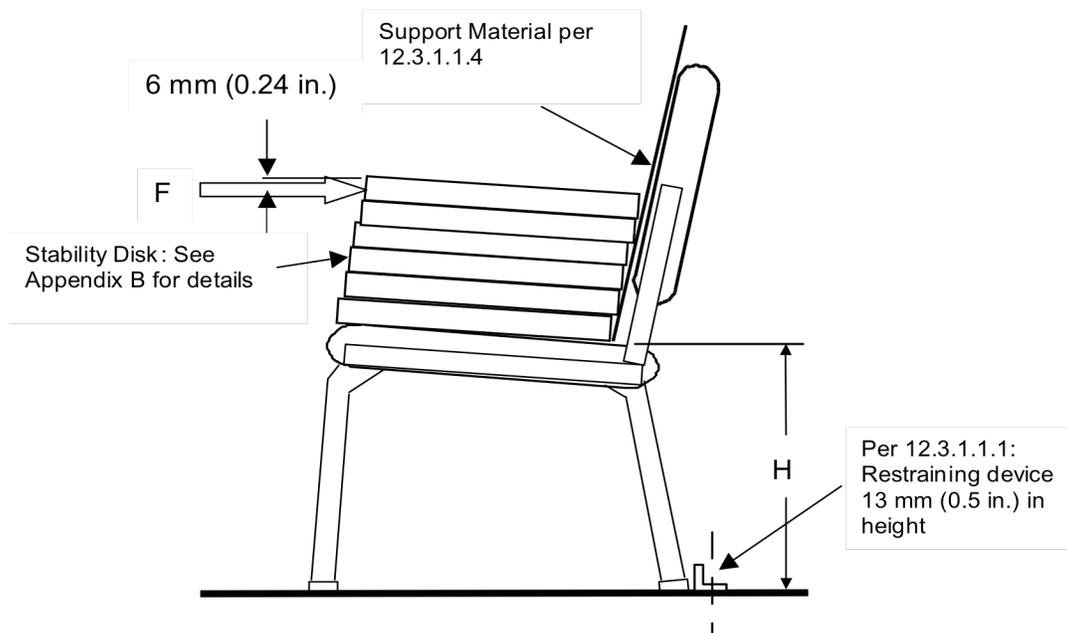
**Figure 12a - Rear Stability Test for Type III Chairs**
