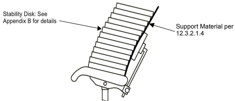
**Figure 12b - Rear Stability Test for Type I and II Chairs**
