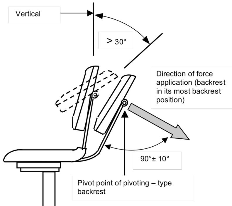
**Figure 6d - Force Application for Backrests that Pivot Greater than 30° Backrest Strength Test - Static - Type II and III**
