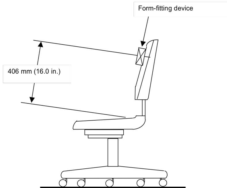
**Figure 15b - Positioning of Form-Fitting Device for Backrests Higher than 452 mm (17.8 in.)
