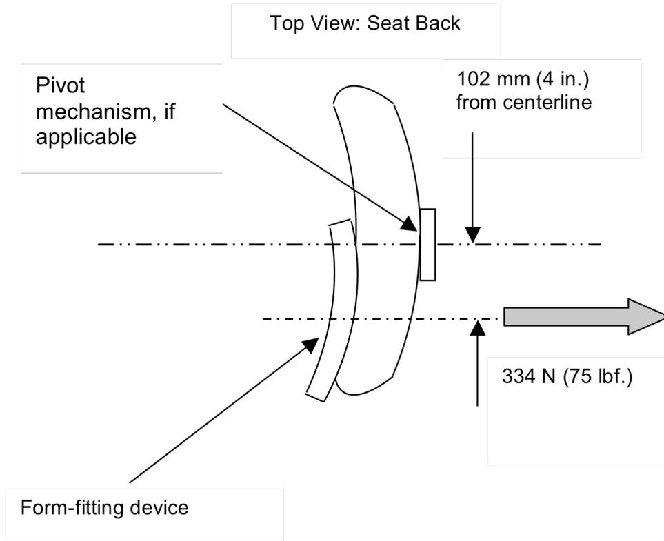
Figure 16f - Off-center Backrest Durability Loading - Left
