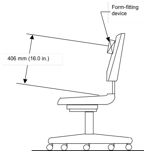
**Figure 5b - Positioning of Form-Fitting Device for Backrests Higher than 452 mm
