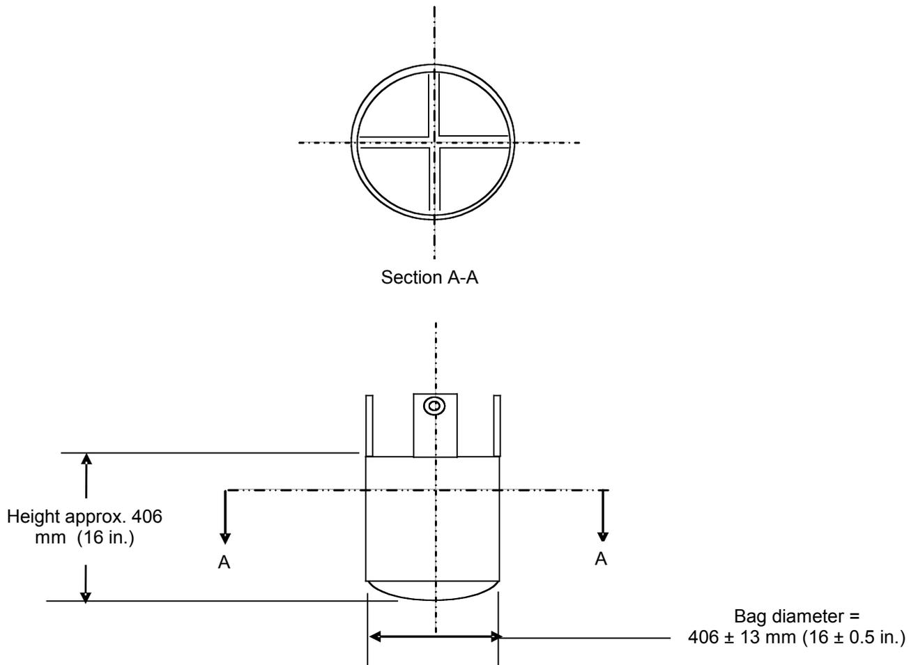
Bag to contain a sufficient quantity of media to bring the bag to the specified load. Media may be shot, slugs, punches, sand, etc. Media may be contained within smaller individual bags/compartments. Media may not be a singular solid material (e.g. single steel or concrete mass).
