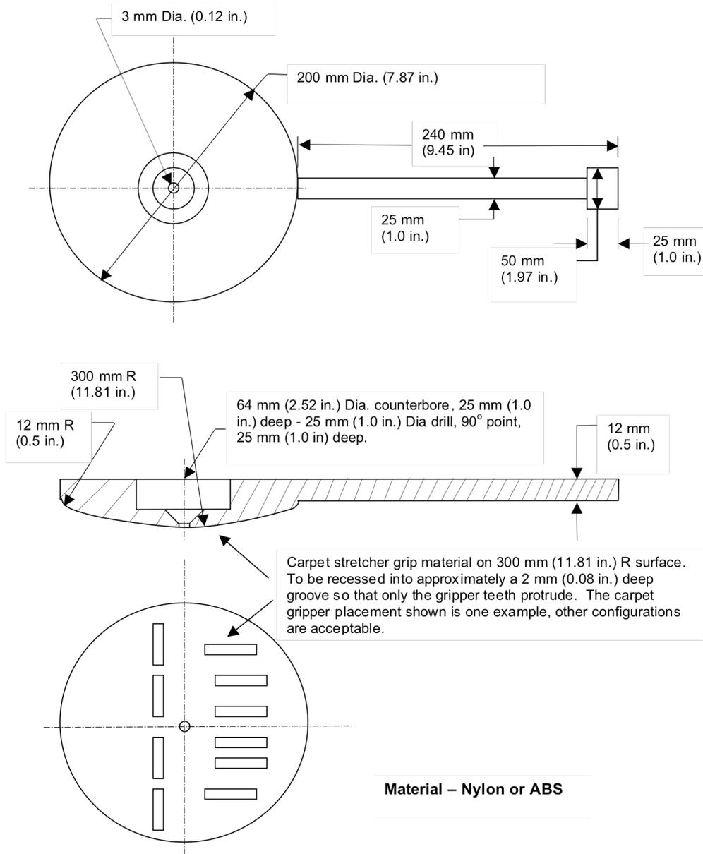
Figure 12e - Front Stability Loading Disk
