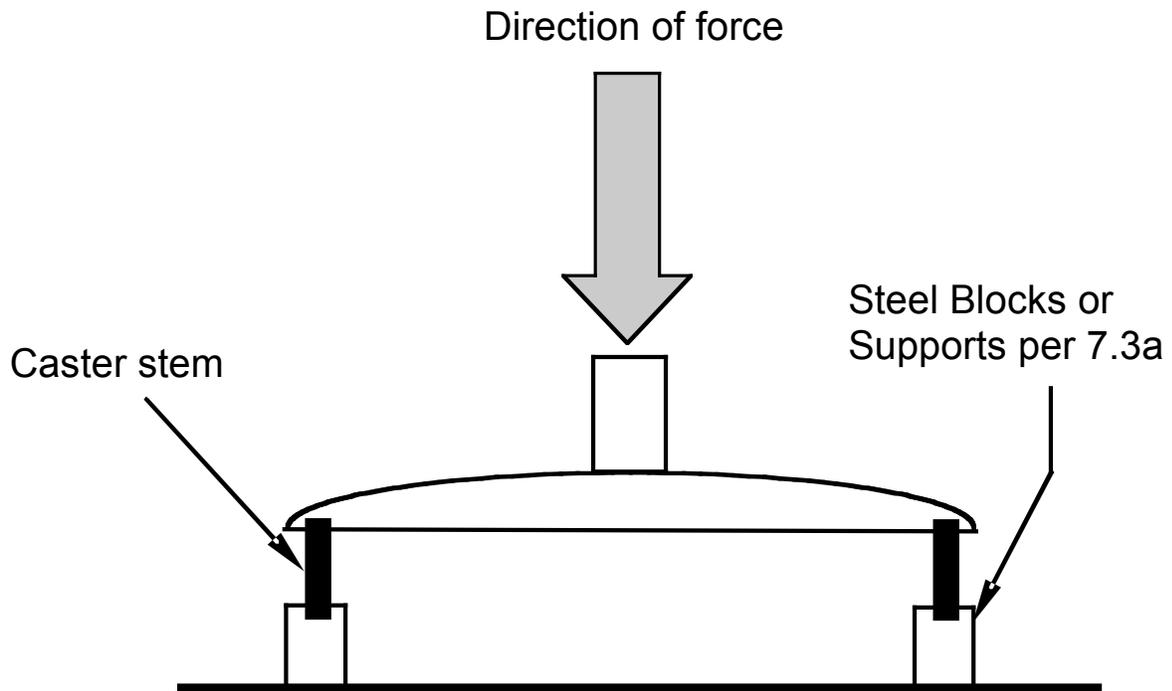
**Figure 7 - Base Test - Static**
