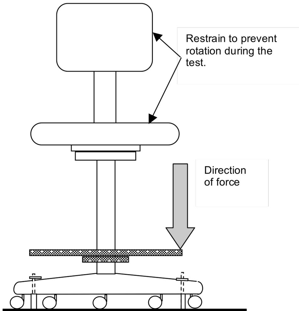
**Figure 20 - Footrest Durability Test - Vertical - Cyclic**
