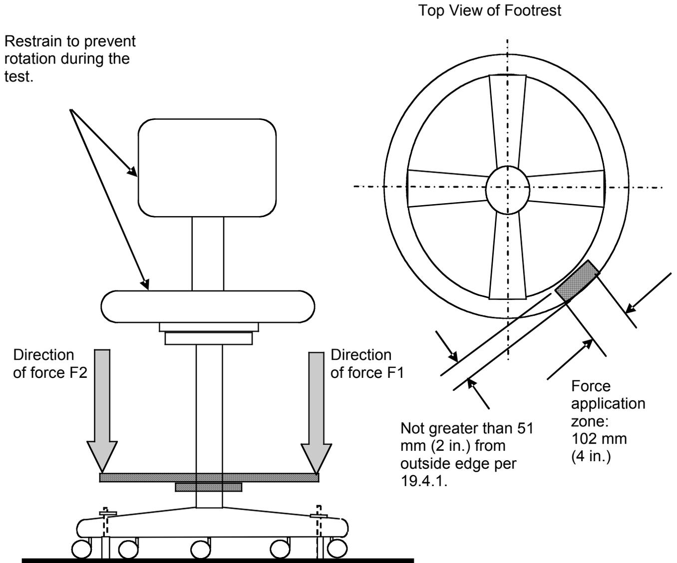
Figure 19 - Footrest Static Load Test - Vertical
