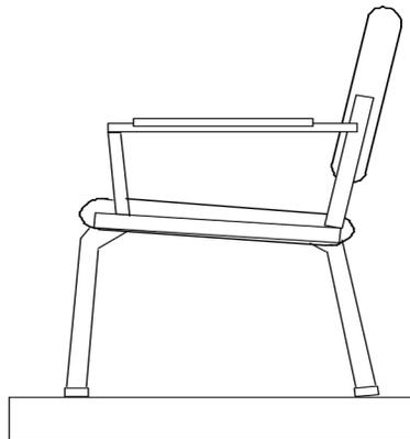
**Figure 4c - Type III - Fixed seat angle, fixed backrest**
