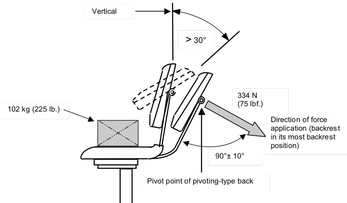
Figure 16d - Force Application for Backrests that Pivot Greater than 30 Degrees Backrest Durability Test - Cyclic - Type II and III
