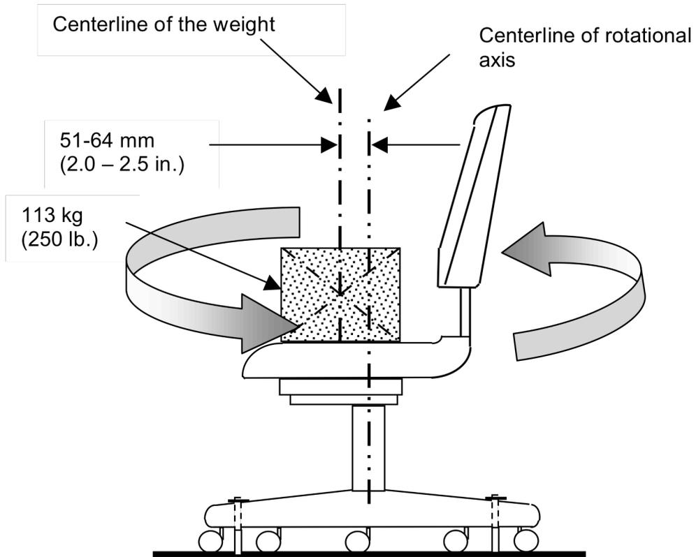
**Figure 9 - Swivel Test – Cyclic**
