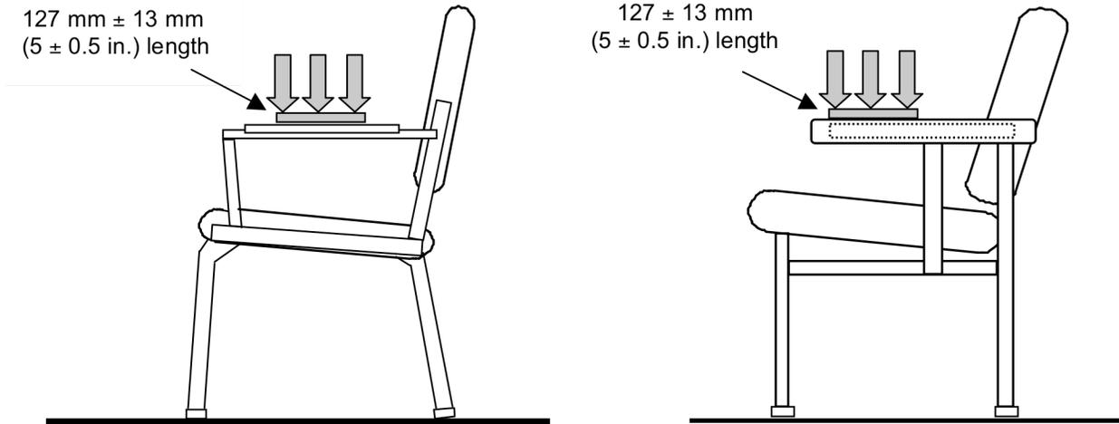
**Figure 13a - Arm Strength Test - Vertical - Static**
