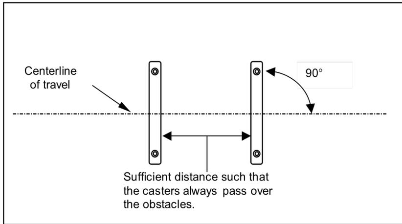
Figure 17d - Obstacle Layout for Chairs with Legs
