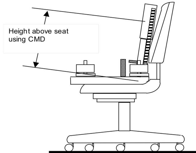
**Figure 6a - Height Determination
