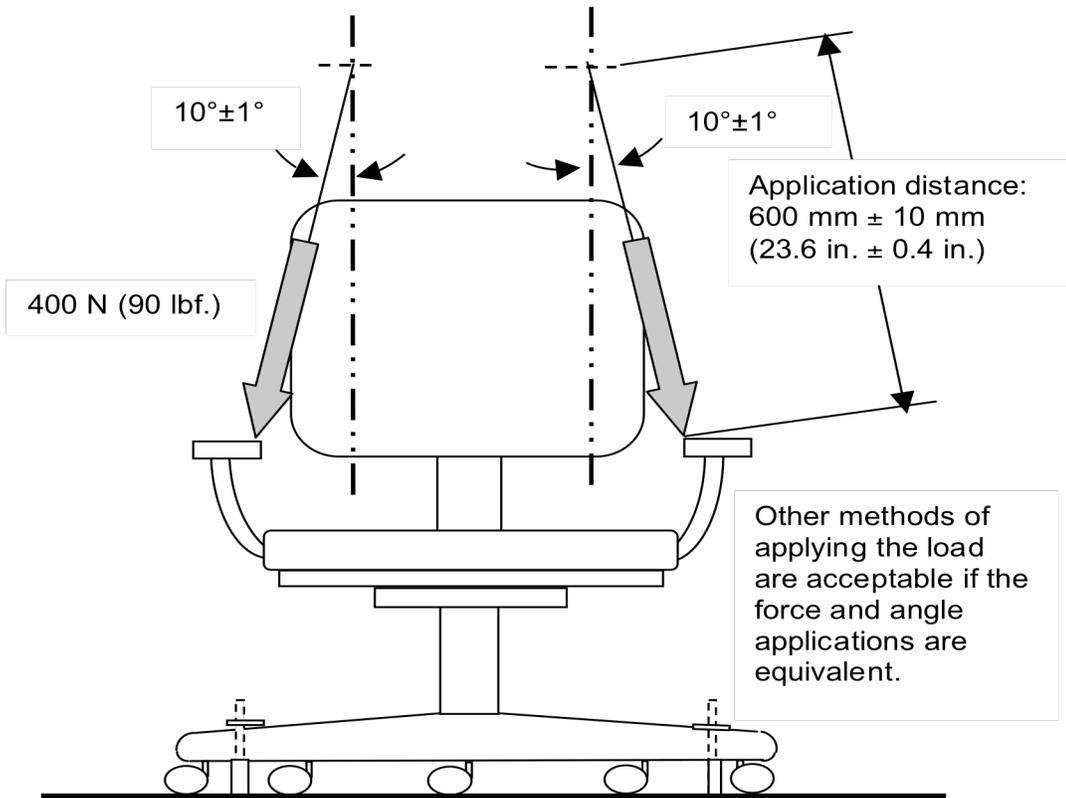
Figure 21b - Arm Durability Test - Cyclic
