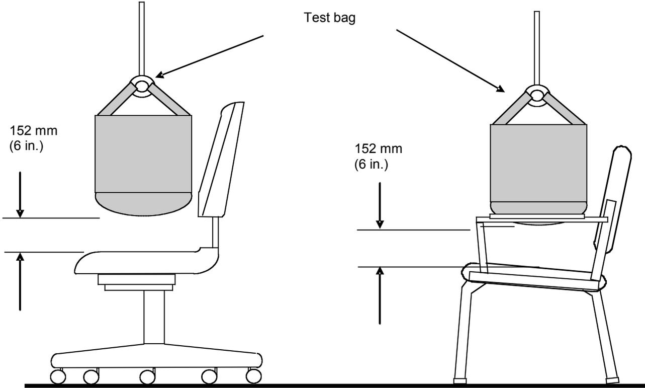
Figure 8 - Drop Test - Dynamic
