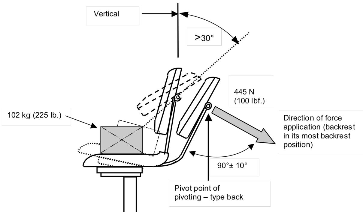
**Figure 15d - Force Application for Backrests that Pivot Greater than 30° Backrest Durability Test - Cyclic - Type I**
