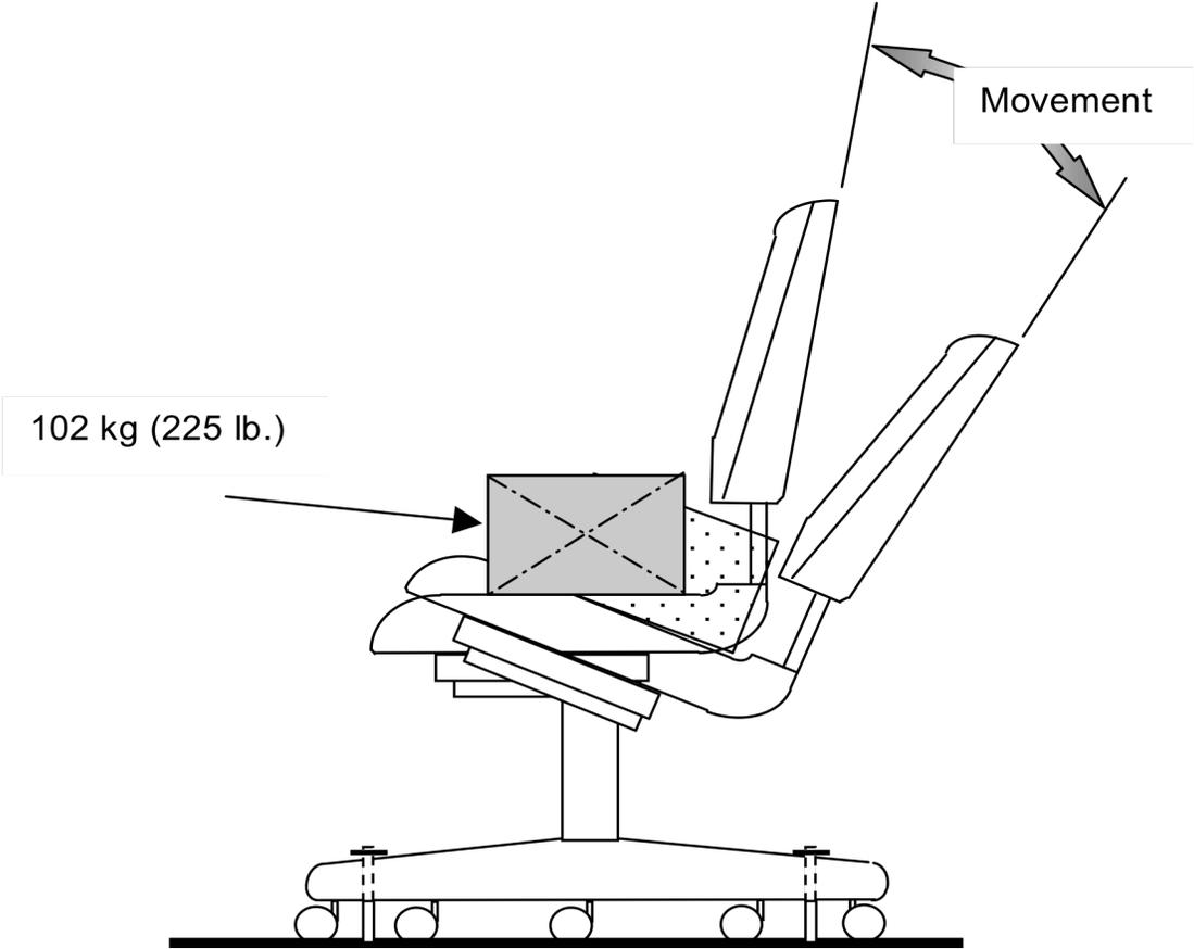
Figure 10 - Tilt Mechanism Test - Cyclic
