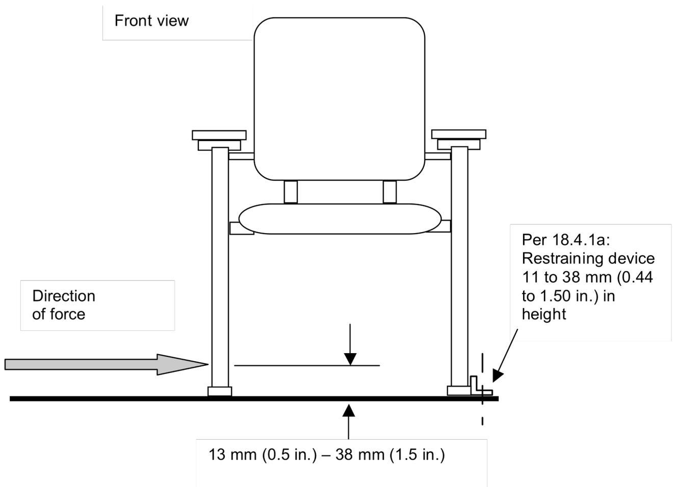
Figure 18b - Leg Strength Test - Side Application
