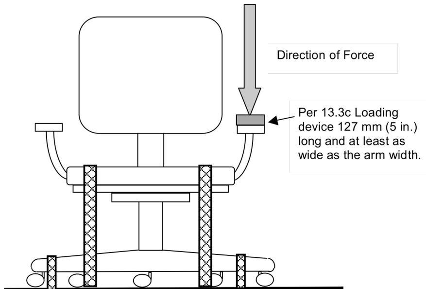
**Figure 13b - Arm Strength Test - Vertical - Static**
