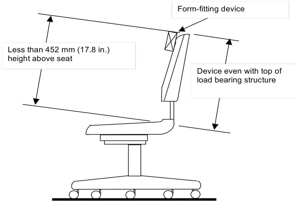
**Figure 5c - Positioning of Form-Fitting Device for Backrests Lower than 452 mm (17.8 in.) Backrest Strength Test - Static - Type I**
