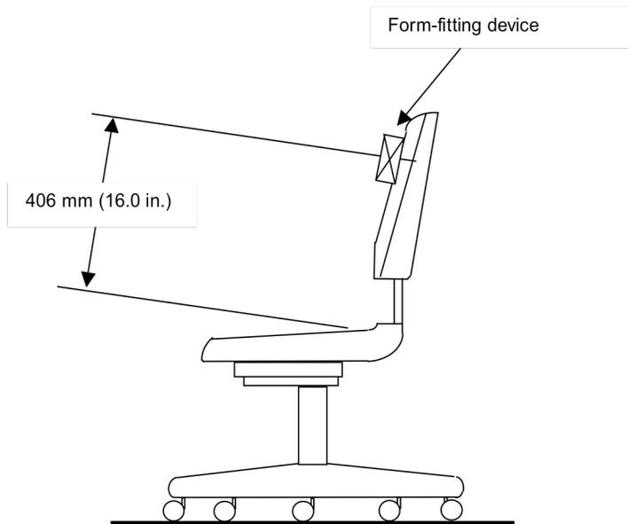
**Figure 6b - Positioning of Form-Fitting Device for Backrests Higher than 452 mm
