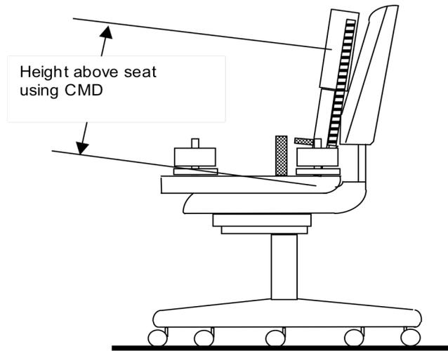
**Figure 5a - Height Determination
