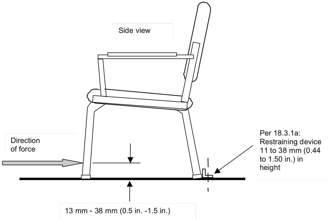
Figure 18a - Leg Strength Test - Front Application
