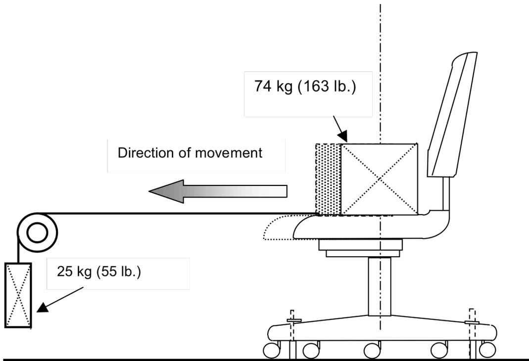
Figure 22 - Out Stop Test for Chairs with Manually Adjustable Seat Depth
