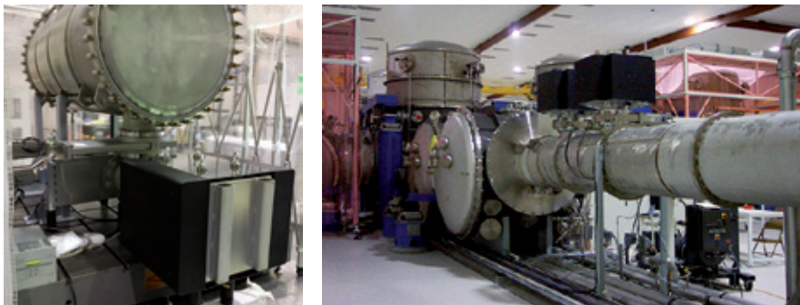
Fig. 16 - Agilent Ion Pumps mounted on LIGO Gravitational Waves Detector and at MIRAPRO for KAGRA Gravitational Wave Interferometer.
