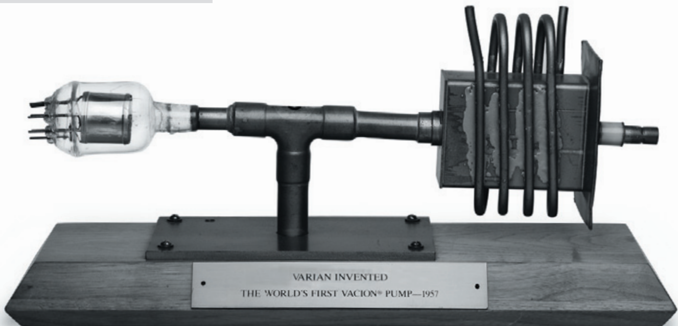
Fig. 1 - The first Vaclon, sputter ion pump was invented by Varian in 1957.
