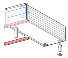
... and slip the supplied rubber bar onto the bottom edge of the front panel.
