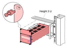
...and fasten the adapter panel to the rack chassis adapter using the screws supplied with the VGC401.
