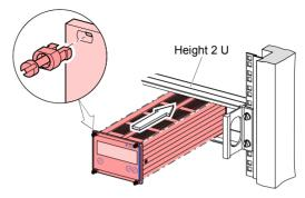
... and fasten the VGC401 to the rack chassis adapter using the screws supplied with it.
