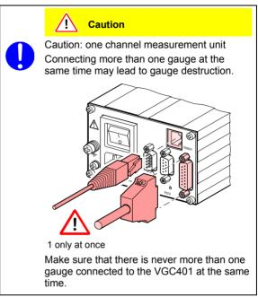
Connect the gauge to one of the two SENSOR connectors on the rear of the unit. Use a screened 1:1 cable (electromagnetic compatibility). Make sure the gauge is compatible ( $\rightarrow \mathbb{R}$  8).
