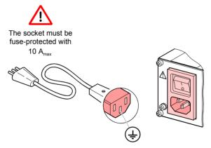
If the unit is installed in a switch cabinet, the mains voltage should be supplied and turned on via a central power distributor.
