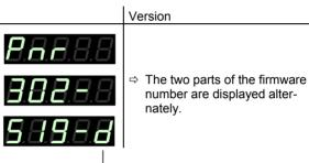
The last character indicates the modification index (-, A  $\dots$  Z). Please mention this index when contacting INFICON in the event of a fault.
