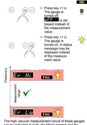
can be activated in both, the Measurement and the Parameter mode ( $\rightarrow \blacksquare 42$ ).
