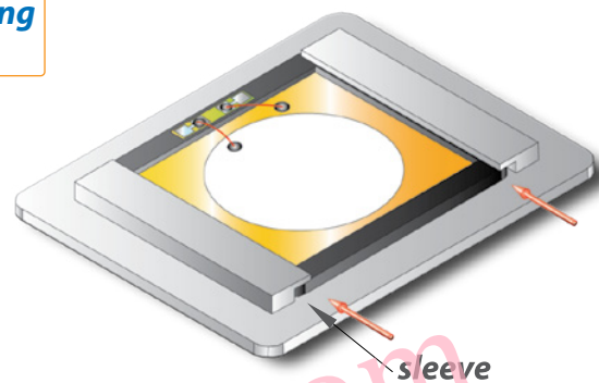
Plastic deformation method (Ultrasonic)
