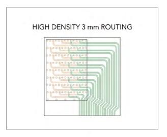
Figure C2: High-density routing with one half the routing layers: one 28 Gbps differential pair per 1.5 mm per layer (3 mm design), and one 28 Gbps pair per 2 mm (2 mm design) results in 33% higher board utilization, 50% layer count reduction and significant PCB cost savings.
