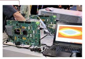
Teraspeed® Consulting demonstration of a 28 Gbps backplane system attaching two Xilinx VCU109 Evaluation Boards across Samtec's ExaMAX® backplane connectors. The demo leveraged advanced design optimization techniques that minimize insertion loss, return loss and crosstalk, while utilizing advanced PCB materials. Photo courtesy of Xilinx.
