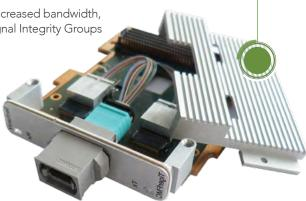
TechWaY TigerFMC, a VITA 57.1 compliant mezzanine card integrates Samtec's FireFly™ with 10 full duplex, 10 Gbps optical links, for 200 Gbps aggregate bandwidth.
