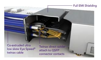
Figure B1: Mechanical Anatomy of Samtec FQSFP
