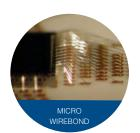
Pitches down to 25 µm on 20 µm pad with complex multi-tiered wirebonds
