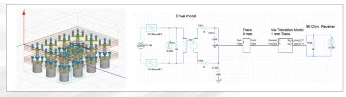
Figure A2: Novel Differential SerDes Package Design Cell Model
