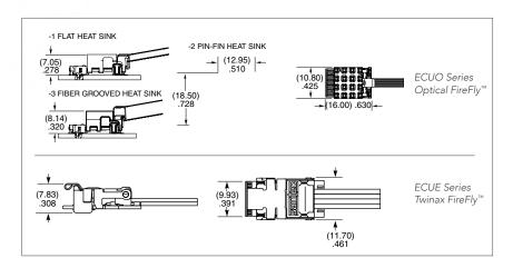
Figure B6: Mechanical Specifications of FireFly $^{\text{TM}}$
