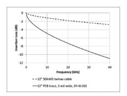
Figure B2: Insertion Loss Comparison of Twinax vs. PCB Traces
