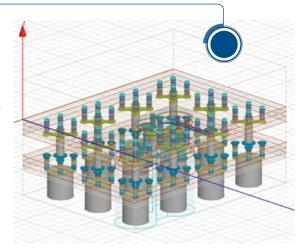
Novel differential SerDes package design cell developed with the IC packaging and signal integrity expertise of the engineers at Teraspeed® Consulting.
