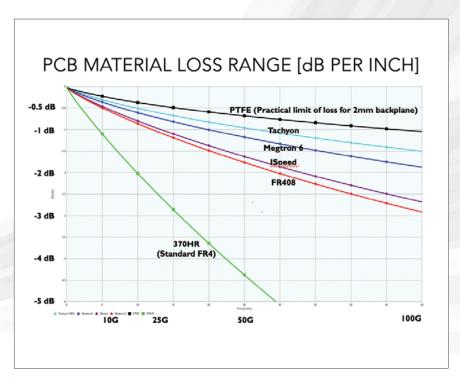
Figure C4: PCB Material Loss Range dB per Inch
