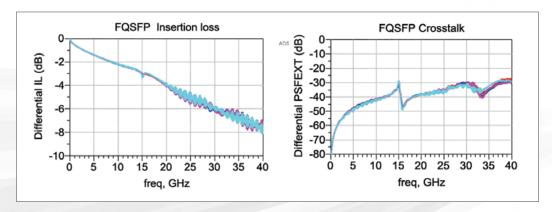
Figure B3: 18-inch FQSFP Cable Assembly Performance
