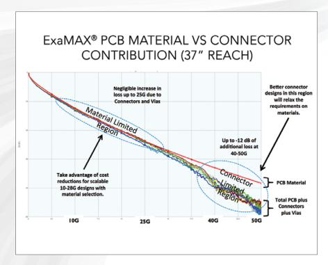
Figure C3: High-speed PCB Material with ExaMAX® High-speed Backplane vs. Connector Contribution
