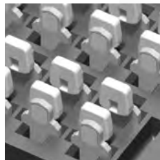
Solder charge terminations (IPC-A-610F & IPC J-STD-001F Class 3)
