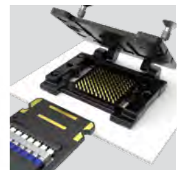
Mating cable for GMI compression array in development (see page 7)
