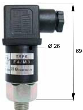
"F4" adjustable pressure switches allow a micro-switch commutation once a preset pressure value is reached. The set point is adjusted working on the central screw (P3 execution) or intercepting the regulation dowel situated inside the instrument, using a 2mm hexagonal key (M2 and M3). Rotating clockwise the set point is increased and vice-versa is decreased. Mechanical stops protect both the spring and the micro-switch from over pressurization.
