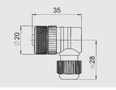
**ZBE 06-02** (4 pole) Right-angled connector with 2m cable M12x1 **ZBE 06-05** (4 pole)
