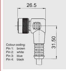
**ZBE 08-02** (5 pole) Right-angled connector with 2m cable M12x1
