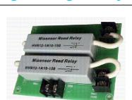
>20KV Reed Relay Photo shows each 2 HV Reed Relays (Model HVR12-1A15-06-150) are installed in a PCB, and breakdown voltage 20KVdc at least.
