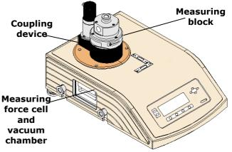
The measuring force cell is associated with an Auto Calibrating Function (see further) which enables to apply to it, easily and whenever it is necessary, a reference force that is equivalent to the product of the mass multiplied by the local acceleration of the gravity ( $F = M \times g$ ) in order to recalibrate it.
