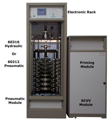
The complete 60000 pressure standard consists of four interconnected systems mounted into two separate standard rack enclosures.
