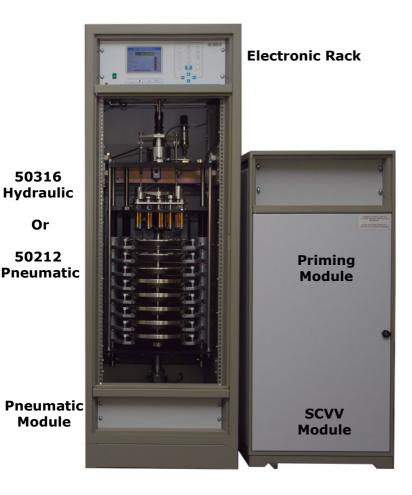
The complete 50000 pressure standard consists of four interconnected systems mounted into two separate standard rack enclosures.
