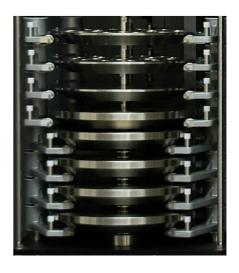
The main masses (from 2048 g up to 16384 g) are loaded / unloaded with three arms linked to a pneumatic actuator. All movement are user adjustable.
