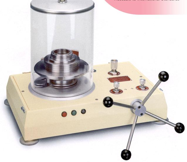
Utilising primary pressure measurement, with accurately calibrated weight masses loaded onto a gas lubricated piston. The weights balance the upward force created by the pressure within the system.
