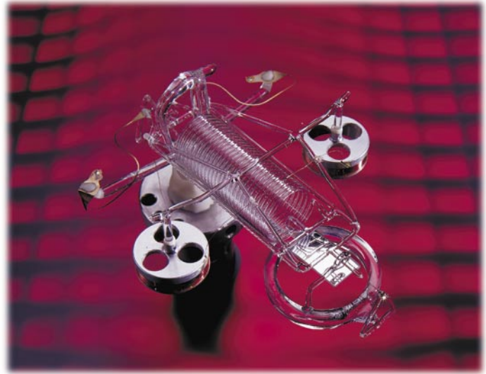
Series 7050's feature Ruska's unique fused-quartz sensor. This rugged transducer offers unequalled precision and a stability of 0.0075% of reading per year.
