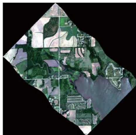
Rectified and georeferenced AisaEAGLE data. Image courtesy of CALMIT, University of Nebraska, Lincoln, NE, U.S.A.
