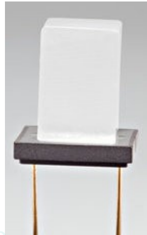
Combination of crystal with a sensL SPM
