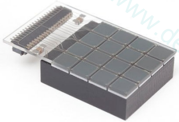
SPMArray2 (glass) 3-side scalable 16 element detector
