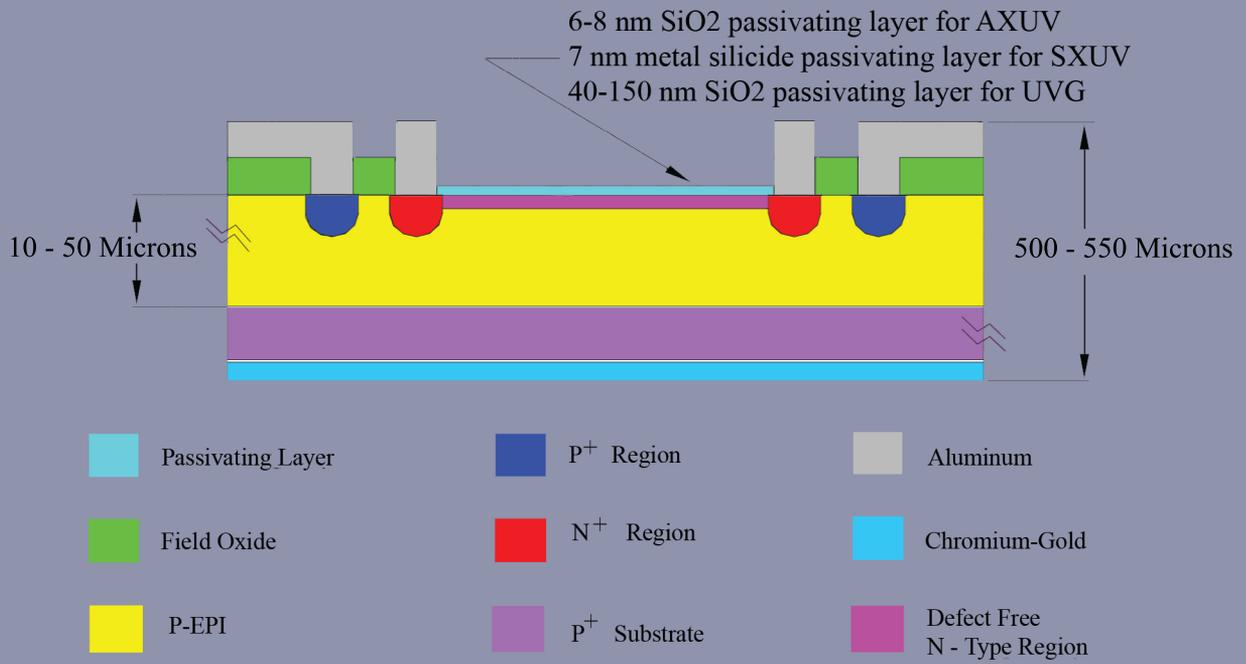
Structure of the AXUV, SXUV and UVG Photodiodes
