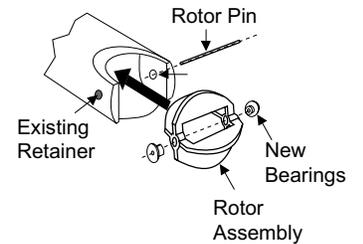
4. Tap the second retainer (rotor pin clearance hole inwards) into the hole while lining up the rotor pin with the center of the retainer hole. This completes the rotor replacement procedure.
