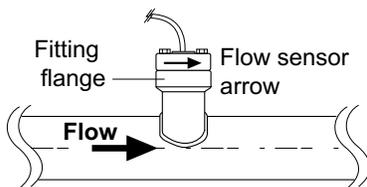
3. Slip two washers onto each bolt and insert the bolt/washer onto each of the four fitting flange holes.
