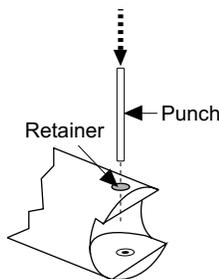
3. Insert the new rotor assembly and bearings into the rotor housing of the sensor and place the new rotor pin (axle) through the open end of the rotor housing, through the rotor and bearings, and into the previously installed retainer.
