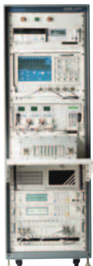
DC to DC Converter ATS
