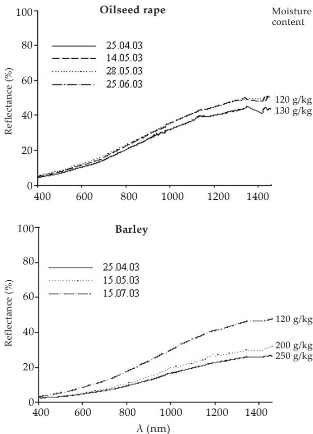
Figure 6. Soil reflectance at different wavelengths ( $\lambda$ ) as affected by soil moisture content of the topsoil (0–20 cm) during vegetation of winter oilseed rape and barley measured with field configuration ( $n = 15$ )
