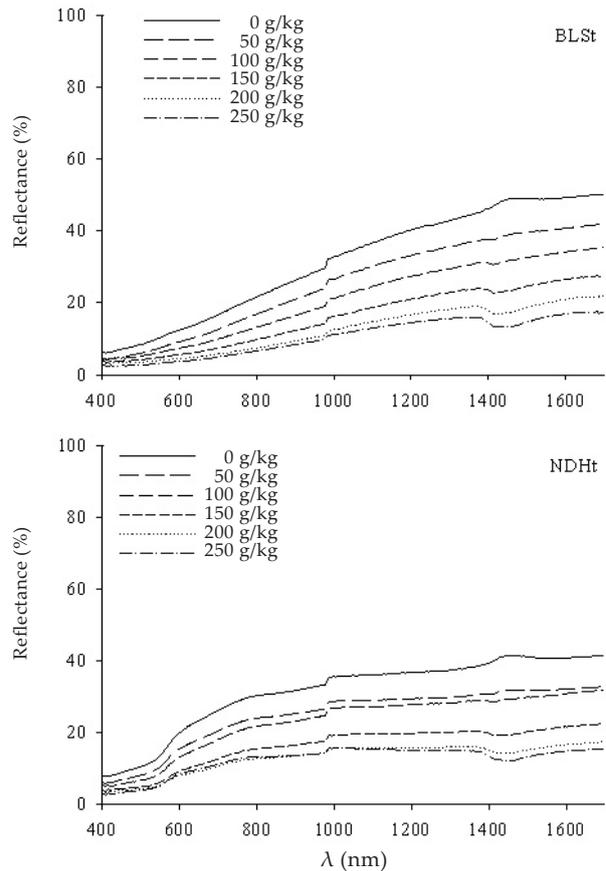
Figure 4. Soil reflectance at different wavelengths ( $\lambda$ ) of two soils as affected by varied soil moisture contents (g/kg) measured with laboratory configuration OMK ( $n = 20$ )
