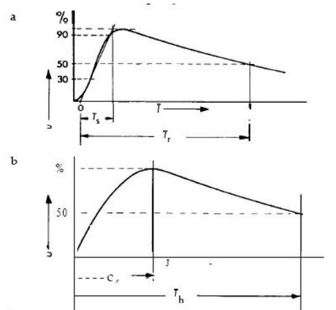
Fig. 4 Standardized test voltages
