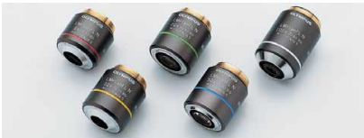
LMPLFLN (-BD) Plan SemiApochromat series The LMPLFLN (-BD) series provides more free space between the objective lens and the specimen than other Plan SemiApochromatic objective lens series so that it can prevent from collision between objective lens with the stepped specimen. Since exit pupil positions from 5x through 100x are standardized, no switching of the DIC prism lever position is necessary when the objective lens power changes. Use the BD series in brightfield and darkfield observation.
