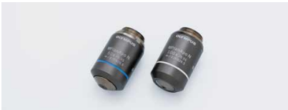
MPLAPON Plan Apochromat series This is a Plan Apochromat objective lens series for brightfield observation with chromatic aberration corrected at high level. Olympus has assured that this series has the optical performance (wavefront aberration) with a Strehl ratio*1 of 95% or more*2 first in the world as a universal objective lens. This series is also compatible with a differential interference contrast or simple polarized observation.
