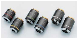
MPLFLN (-BD) Plan SemiApochromat series These Plan SemiApochromat objective lenses completely eliminate chromatic aberration at high level, which is perfect for a wide range of microscopic methods including brightfield darkfield, fluorescence, Nomarski DIC and simple polarized observation. Since exit pupil positions from 5x through 150x are standardized, no switching of the DIC prism lever position is necessary when the objective lens power changes.
