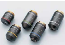
MPLFLN (-BD) Plan SemiApochromat series These Plan SemiApochromat objective lenses completely eliminate chromatic aberration at high level, which is perfect for a wide range of microscopic methods including brightfield darkfield, fluorescence, Nomarski DIC and simple polarized observation. Since exit pupil positions from 5x through 150x are standardized, no switching of the DIC prism lever position is necessary when the objective lens power changes.
