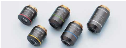
LMPLFLN (-BD) Plan SemiApochromat series The LMPLFLN (-BD) series provides more free space between the objective lens and the specimen than other Plan SemiApochromatic objective lens series so that it can prevent from collision between objective lens with the stepped specimen. Since exit pupil positions from 5x through 100x are standardized, no switching of the DIC prism lever position is necessary when the objective lens power changes. Use the BD series in brightfield and darkfield observation.
