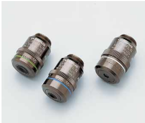
LCD objective lenses (The new correction ring method provides adjustable glass thickness in 0 through 1.2 mm for 20x, 50x and 0 through 0.7 mm for 100x.)
