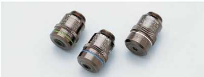
LCPLFLN-LCD series The perfect objective lenses for imaging specimen through glass plate like an LCD application. Aberration correction matched to the glass thickness is possible by using a correction ring.
