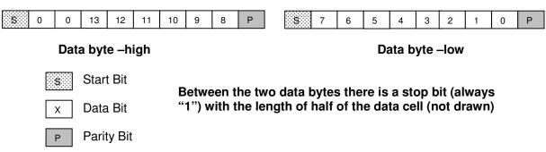
The transmission speed depends on the update rate and ranges up to 8 KHz.
