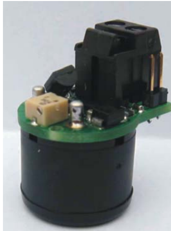
Fig. 1 ECO-Sure CO sensor + 4-20 mA p.c.b.
