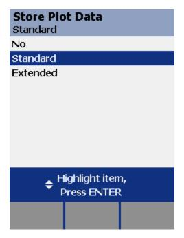
'No' will mean that no plot data is stored. 'Standard' will store plot data and 'Extended' will store plot data to 350 MHz. This is also true if category 6 is selected. When class F and 'Extended' are selected, the test will run to 900 MHz.
