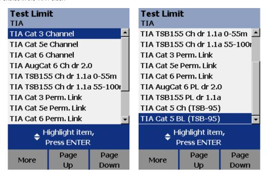
TIA TSB-155 CH dr 1.1a is a channel measurement designed to verify the performance of an existing category 6 cabling system for 10GBASE-T operation. The same is for TIA TSB-155 PL dr 1.1a.
