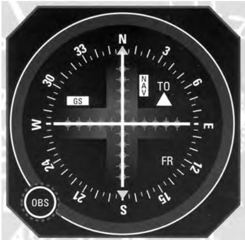
Combined OBS (Omni Bearing Selector) and CDI (Course Deviation Indicator)
