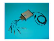
The TEMP14 is a highly exact temperature gauge measuring instrument for the most different areas of application. By the compact construction method and driver-free installation the TEMP14 is applicable very adaptably. With his 16 measuring channels and the different precision temperature sensors varied Applications can be realised in the temperature metrology.
