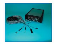
The precision temperature gauge TEMP12 is an electronic gauge for the temperature measurement. The device is based on a module system. A variety of ranges of application arises from it. These variants are different with respect to the port connected to a computer, the power supply unit, the number of available measuring channels and the design of casing.
