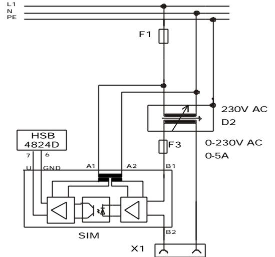
The SIM converts the load current into a voltage signal. The load current is digitally displayed using the HSB4824D.
