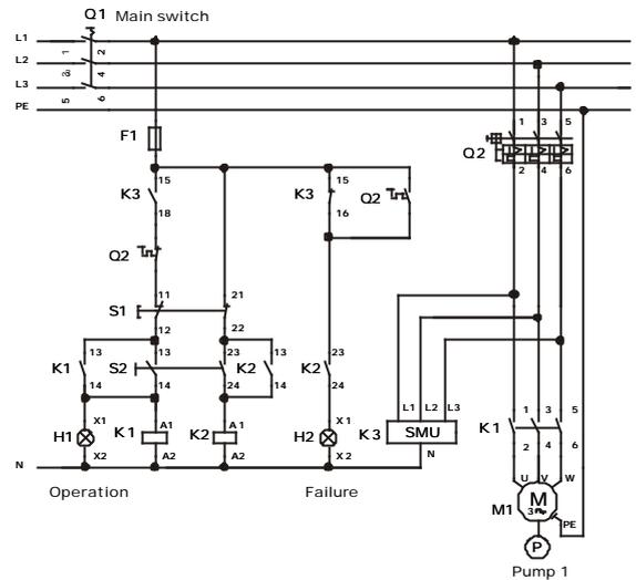
The SMU monitors a pump motor for over voltage.
