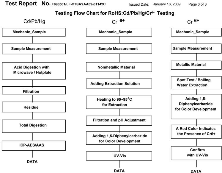
The samples were dissolved totally by pre-conditioning method according to above flow chart for Cd,Pb,Hg.
