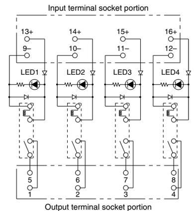
Note: Cannot be equipped with Power PhotoMOS standard type relays. However, equipping with voltage sensitive type of Power PhotoMOS relays (AQZ○○OD) is possible.
