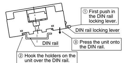
3) To remove the unit from the DIN rail, use a flat head screwdriver to pull out the DIN rail locking lever.
