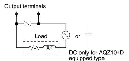
4) Even if spike voltages generated from the load are limited by a clamp diode or R-C snubber, inductances in long circuit wires will still create spike voltages. Keep wires as short as possible to minimize inductance.
