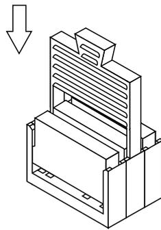
(2) Pull the removal key up to remove the module.
