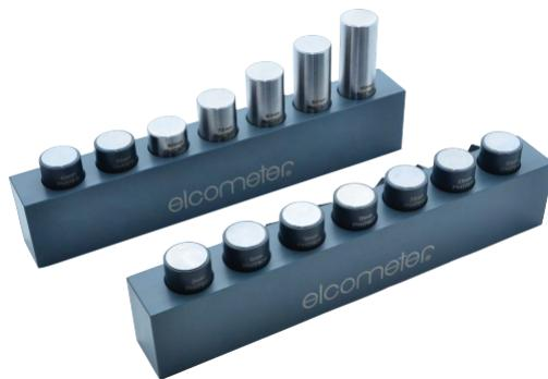
Calibration standard sets and individual standards are supplied complete with calibration certificate.
