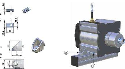
Important: The grooves of the sensor housing, the nuts and brackets are compatible to the aluminium building kit system from *item Industrietechnik GmbH* (www.item.info).
