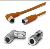
Mating Connector M12, 4 poles, shielded straight, M12 for self assembly D4-G-M12-S D4-W-M12-S angular, M12 for self assembly protection class: IP67 temperature: -25...+90 °C cable passage: ø 4...8 mm wire cross-section: 0.14...0.34 mm<sup>2</sup> mode of connection: spring cage
