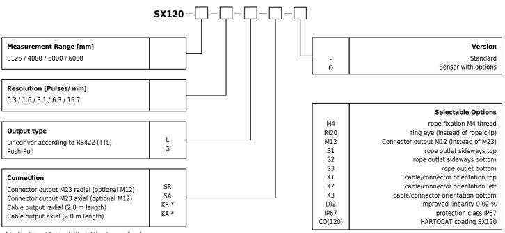
\* for linedriver: 10 wires (with additional sensor lines) for push-pull: 8 wires (without additional sensor lines)
